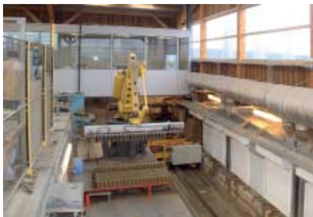
Beladung der Trocknerwagen und Transfer in den Trockner Loading of dryer cars and transfer to the dryer
